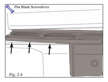
(d) Lightly pull up on the bumper inner cap and from the underside of the bumper, press the tabs holding the cap in place. Use a large flat blade screwdriver when pressing the tabs inward (Fig. 2-4).
