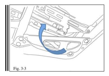
(d) Remove the factory bracket by rotating and moving it towards the centerline of the vehicle (Fig. 3-3).
