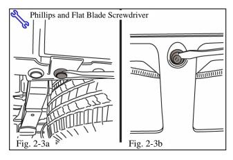
(c) Remove the plastic plug holding the bumper cap onto the lower portion of the bumper (Fig. 2-3a). Remove the plug behind the license plate in the center of the bumper using a Philips screwdriver to remove the plastic pin (Fig. 2-3b).
