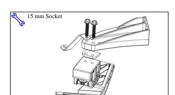
(2) Torque the fasteners from Step 1 to 44 N·m (33ft-lbs) (Fig. 6-2).
